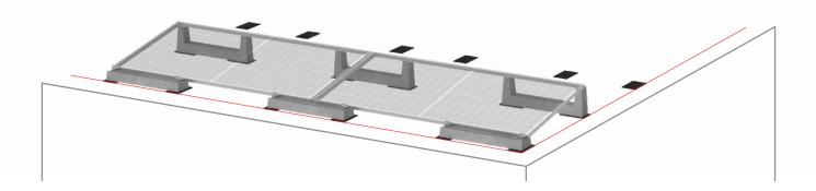
Position the third row of ballasts (EV) aligned with the membranes.
