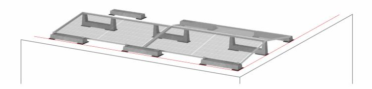
Secure the first panel of the second row on the EP ballasts using clamps 23900/PWC.EP.
