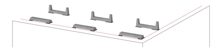
Position the first row of panels, aligning the sides of the frame with the grooves on the ballasts. Check that the corner of the modules coincides with the centre of the EV ballasts, and is halfway along the EP ballasts
