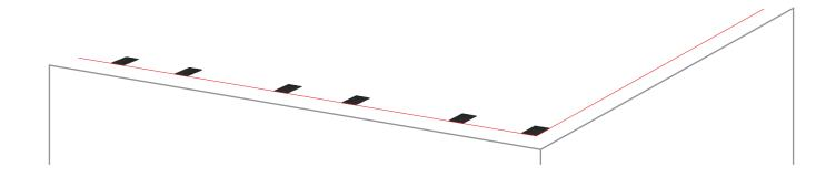
Place the first row of EV ballasts on the membranes. The spacing between the structures should be such that each ballast – except for the end ones – is halfway between two panels.
