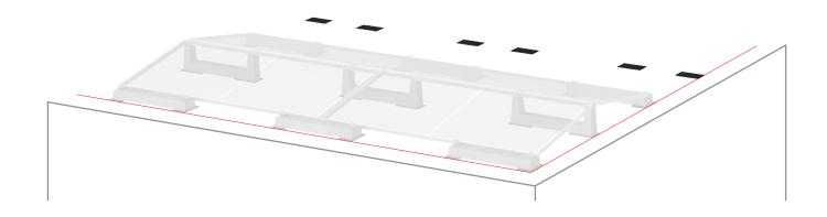
Position the fourth row of ballasts (EP) aligned with the membranes.
