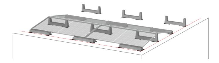
Place the first panel of the third row aligned with the grooves on the ballasts. If necessary, adjust the spacing between the structures, bringing the frame flush against the ballasts.
