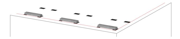
Place the EP ballasts aligned with the membranes, checking for correct alignment with the structures of the structures of the previous row.
