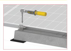
Position the third row of membranes, checking for alignment and placing them in the same direction as used for the first row (EV ballasts).
